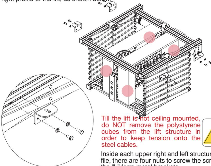
The drawing below indicates the recommended position where to mount the “L” form metal brackets. In this installation manual, we suppose an installation to a flat and horizontal ceiling made of concrete.
