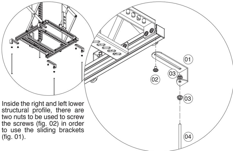
Inside the right and left lower structural profile, there are two nuts to be used to screw the screws (fig. 02) in order to use the sliding brackets (fig. 01).
