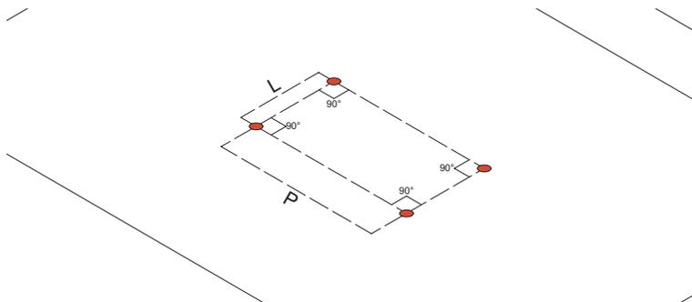
Now drill the holes in the ceiling in order to fix the brackets.
