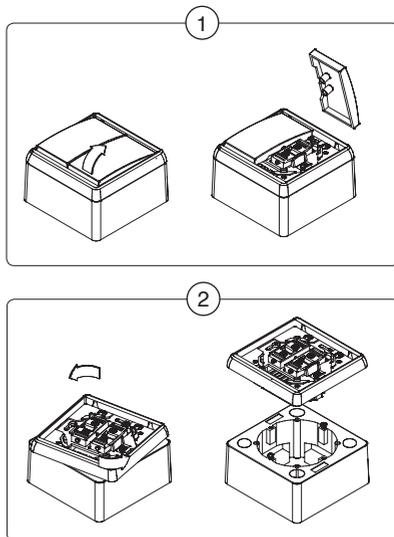
Fig. 1 Without using screwdrivers, remove the up/down buttons.
