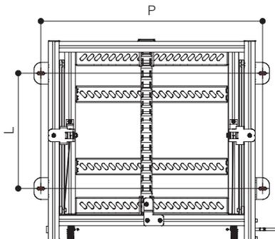
Mark these measures onto the ceiling, in the required position, taking care to keep the squareness between the four points.
