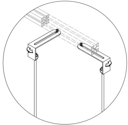
After fixing the threaded bars (fig. 04) and defined the right length, the false ceiling plate can be mounted using two types of screws.
