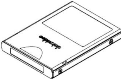
3. After the SSD/HDD is placed back into the enclosure and the four screws are screwed, the SSD/HDD enclosure will be shown as the diagram.
