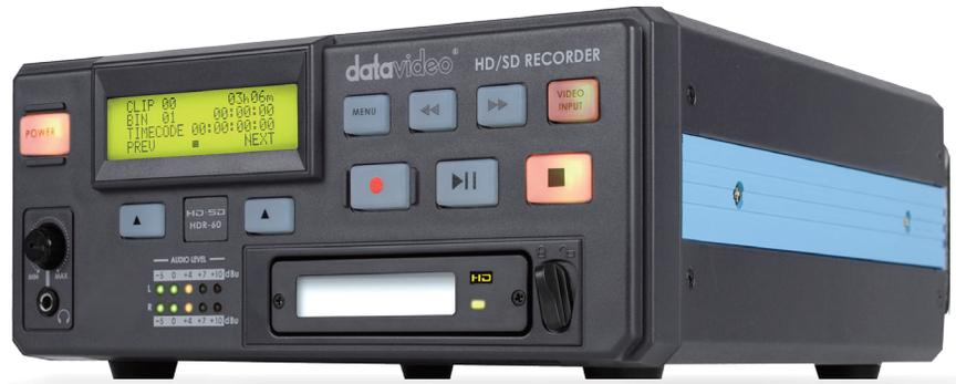
The Datavideo HDR-60 is a portable desktop HD video recorder & player, with a removable enclosure for 2.5" hard drives. The HDR-60 records from standard and high definition video equipment via SDI, with a convenient loop through. RS 422 and 232 remote control interfaces are standard.
