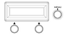
**Press the MENU button to enter the MENU.** The RMC-185 status or the setup menu options are displayed on the LCD panel.
