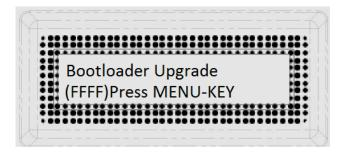
9. Press the MENU key to start the firmware upgrade and do not disconnect the power before the upgrade is complete.
