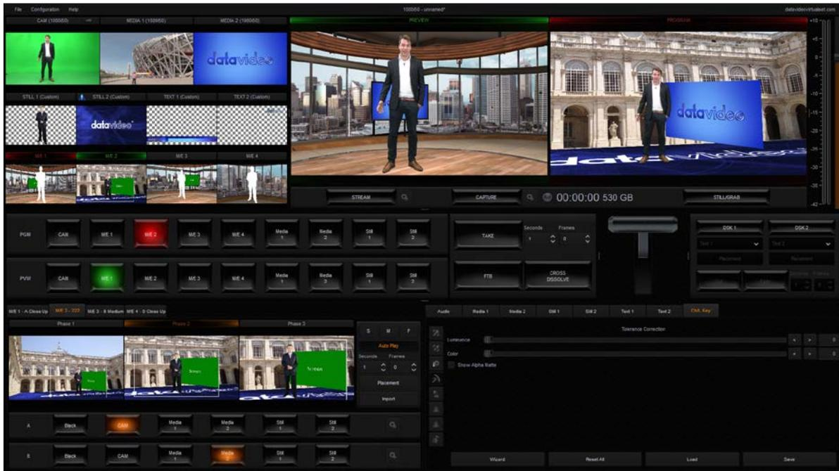
Once the virtualset is imported into the production live module, you can preview your virtualset in the PVW screen. Configure your virtual studio in the Virtual Studio Configuration Panel. Each phase corresponds to a virtual camera position. The user can switch between phases by clicking on phase windows, which is similar to the “cut transition” effect on a switcher.
