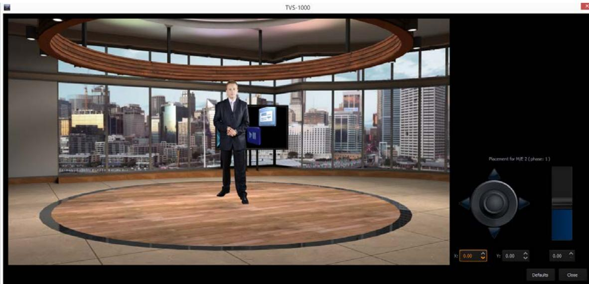
Locate the control panel on the right of the “**Placement Configuration Window**”. X and Y are the adjustable coordinates. The user can use the joystick to configure the PAN and TILT settings. The zoom slide bar on the right adjusts the zoom in/out values accordingly. The user can also use the mouse scroll wheel to adjust the zoom in/out values.
