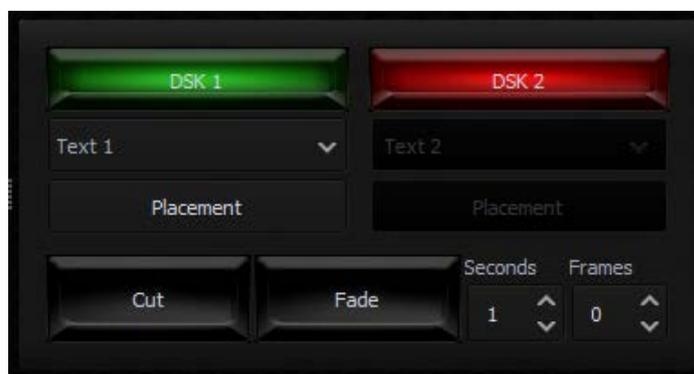
To configure position and size of the downstream key, click on the placement button to open the window shown below.
