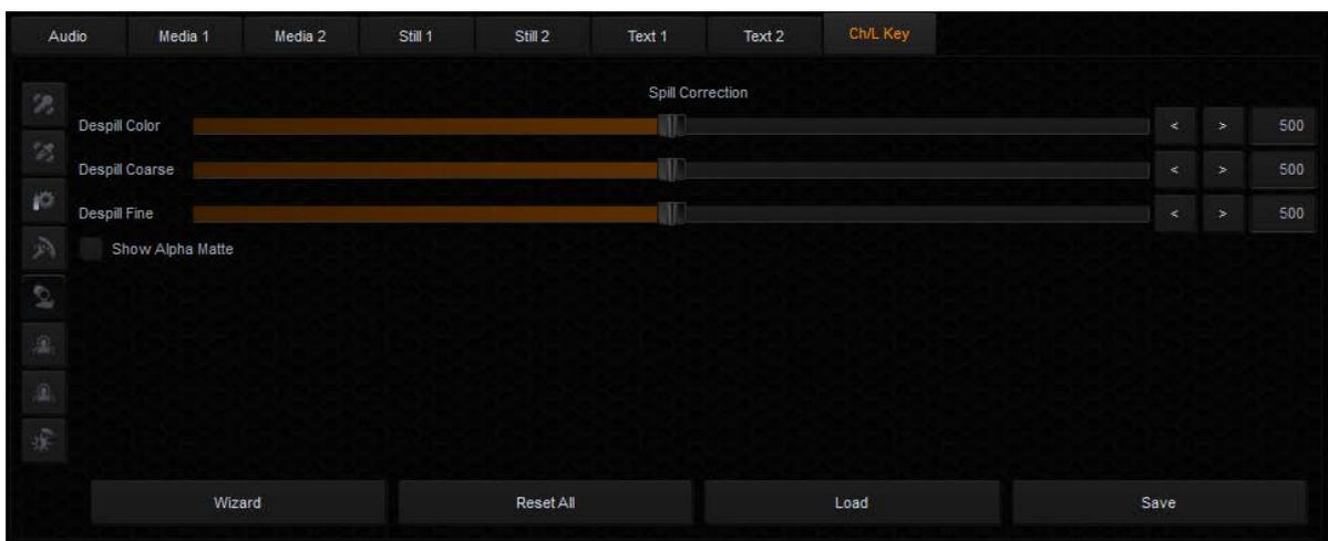
**Despill color** and **Despill coarse** belong to the functions for the preliminary elimination of unwanted colours, and are based on the RGB space.
