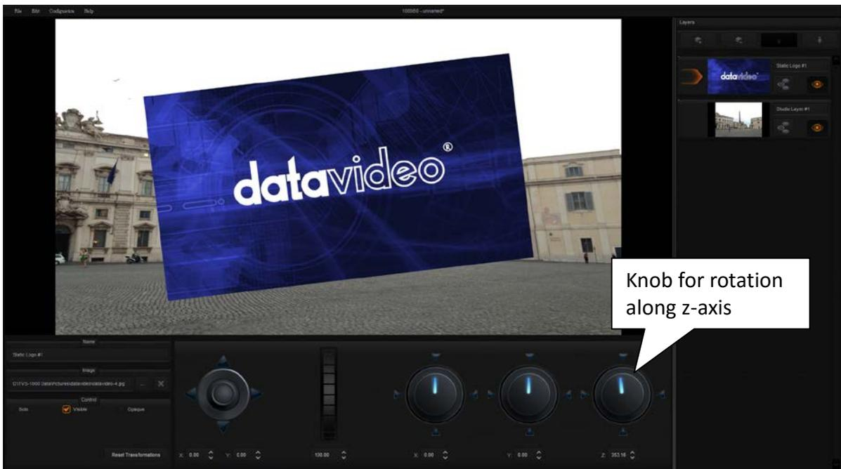
Finally, use the position knob to move the datavideo logo to the desired position and the zoom slide bar to fine-tune the logo to an appropriate size. The diagram below shows you the final work with the floor covered with datavideo logo.
