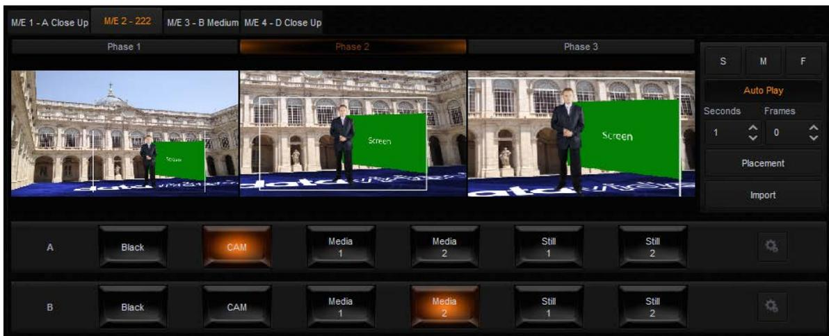
The virtual studio configuration panel is located at the bottom left-hand corner of the screen. Two rows of buttons located below the three phase windows serve the purpose of allowing the user to select talent material source and green screen material source. As depicted in the diagram above, row A is for talent material source selection and row B is for green screen material source selection.
