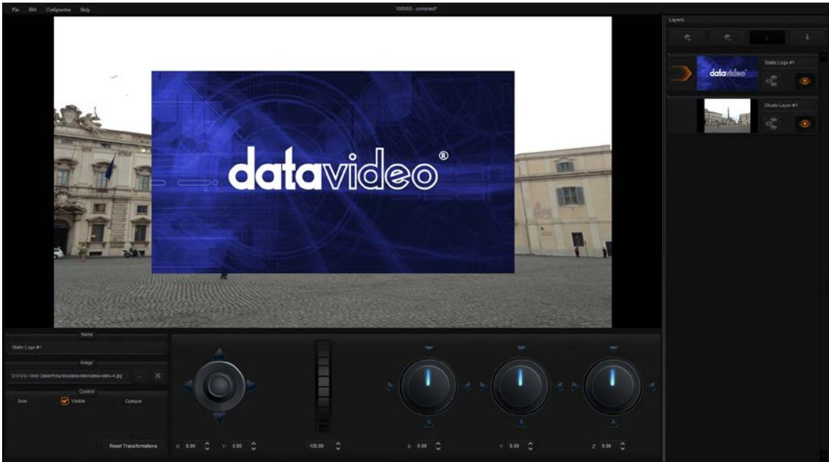
VIRTUALSET maker gives the user the capability to manipulate the layer orientation. Once the logo is imported, you will see that the controllers in pane 3 are enabled. The example below illustrates how you can zoom, rotate and position a “datavideo” logo using the five controllers outlined as follows. The goal is to pave the ground with datavideo logo.
