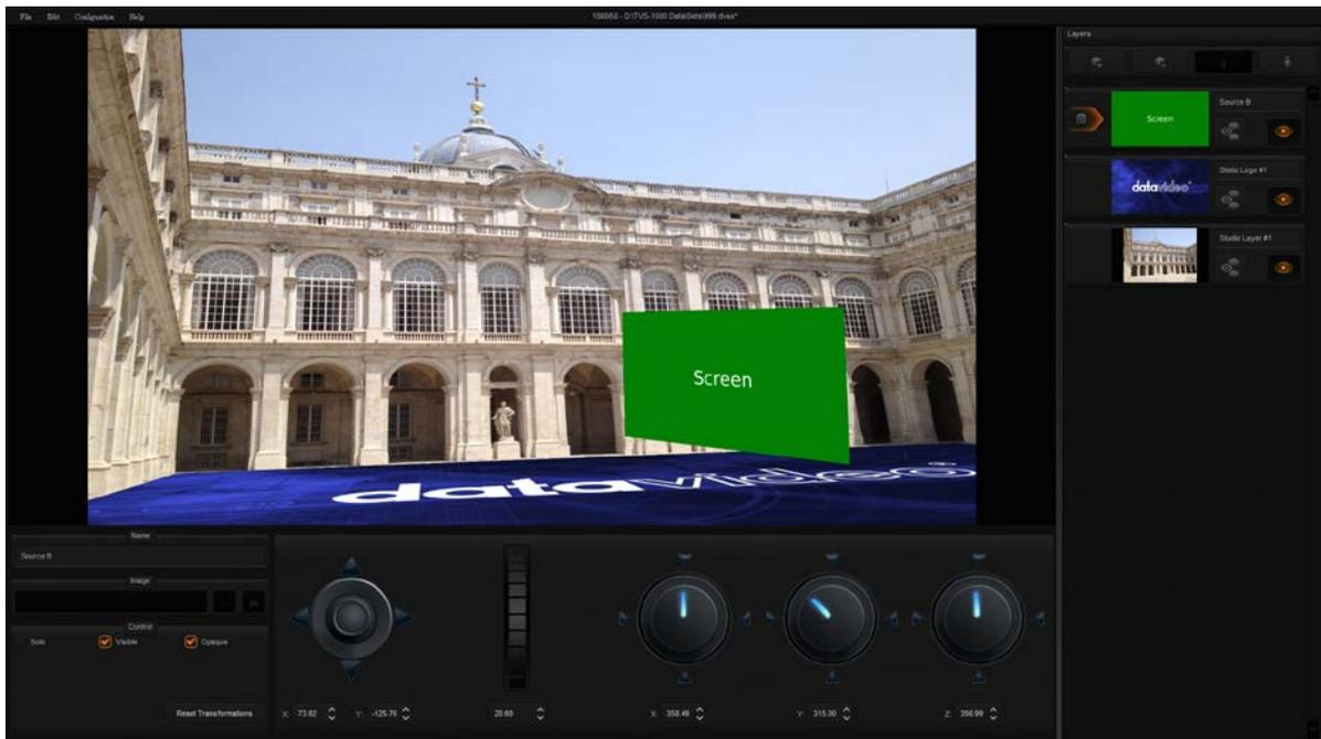
Please note that the Virtualset Maker allows the user to place up to **six screens** on the studio layer. Once all six layers are selected, Source B option will then no longer be visible in the “**Select layer type**” dialogue box.
