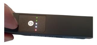
A total of five LEDs are representing the remaining capacity, each represening 20% charge.
