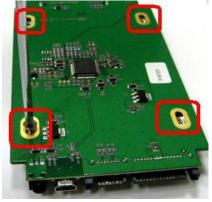
3. Push PCB into the HDD rack
