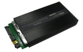
4. Assemble two screws to fasten HD rack rear cover
