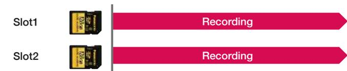
Identical data is recorded onto cards in both slots in this dual recording mode.
