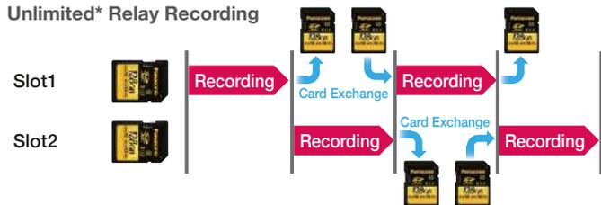
Automatically records continuously from Slot 1 to Slot 2. By changing a full SD card with a new SD card, images can be recorded continuously for many hours.
