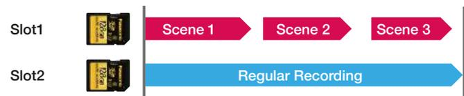
Records ordinary Rec Start/Stop-controlled data in Slot 1, and records all data, even when Slot 1 is stopped, in Slot 2.
