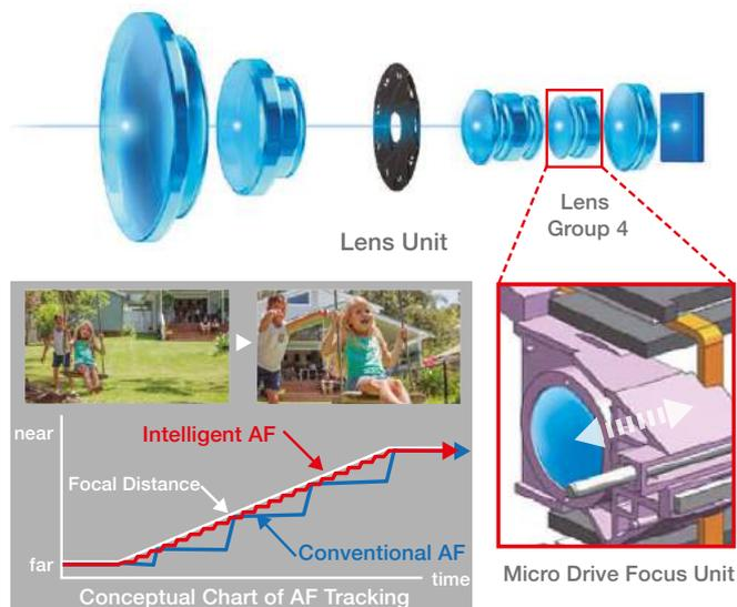
By moving the Micro Drive Focus Unit minutely and quickly, highly precise AF performance is also achieved when shooting in 4K or shooting with a shallow depth of field.
