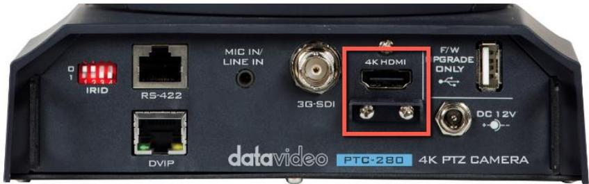
Connect the HDMI OUT to an external connected monitor using an HDMI cable.
