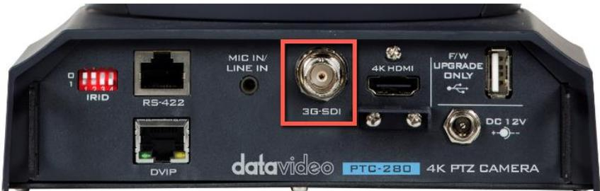
Connect the SDI OUT to an external connected monitor using an SDI cable.
