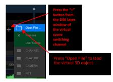
b. Binding the AR virtual object with the Tracker: After the AR object is loaded, please click the object name which is located below the corresponding DSK overlay window for showing the object. After that, please click the cross-shaped icon which is located at the title column. And then the controlled object of the "Offset Adjustment Board" area will change to the AR object of current DSK overlay layer.
