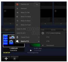
**DDR 1/2/3:** The local video files which need to be played can be added into the lists of the DDR 1/2/3 categories. Please press the "Plus" button on the bottom left side of the window of the list to select multiple video files and to load them into the list of one DDR category for one time.
