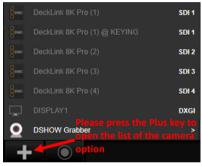
Each time when the plus button is pressed by users, the latest signal sources that can be used by users will be updated immediately. So, for the NDI signal and the signals for the newlyinstalled capturing card, users can press the "Plus" button to update the latest signals that can be used. The signals which are already added into the "CAMERA" category will not be shown again.
