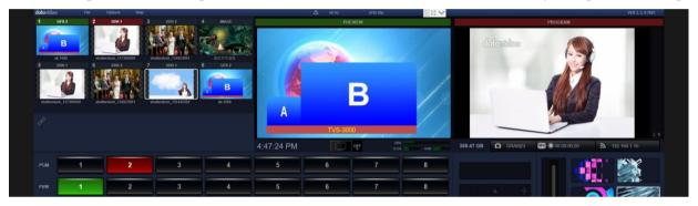
Please select the 8<sup>th</sup> switching channel(If the channel is surrounded by the white rectangular, it means that this channel is selected). After that, please click the "Link" icon which is located on the left side of the switching channel and then please select "Channel" from the dropdown menu. The channel setting row is located below the switching channels. All of the channels will be shown in the channel setting row.
