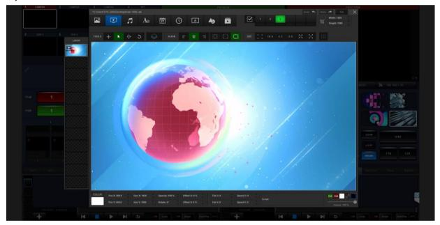
If users want to set a window which provides the main system signal in the virtual studio and to set another window for showing the news broadcasting, users can click "A" at first and then try to drag another window for quoting the signal of other channel. After that, please do the same operations for creating a "B" window.
