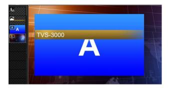
Users can assign current layer for control by clicking the thumbnail of a specific layer. Moreover, users can control the overlay sequence, showing and hiding of the layers by the pop-up menu after right-clicking a specific layer. Users can also press and hold the shift button to click multiple layers to select many layers at the same time for adjusting the location and angle simultaneously.
