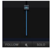
Users can adjust the volume level of a specific channel by dragging the slider. Press the "FOLLOW" button will keep transmitting the audio of the audio for a specific channel to the PROGRAM channel. If the "MUTE" button is pressed, the audio of this channel will not be output to the PROGRAM channel. If the "SOLO" button is pressed, only the audio for the specific channel will be output and the audio output for all other channels will be turned off.
