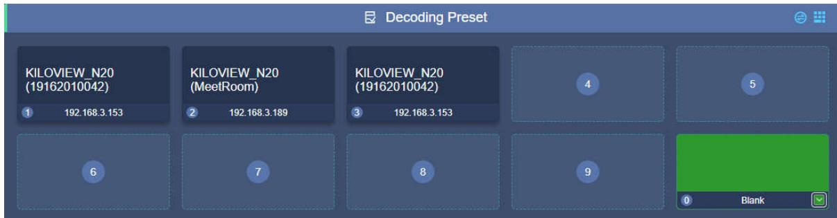
There is a blank output box in decoding preset, if switching to a source without video output, the device will output the set color. It can also be used for testing the output to the monitor by choosing a different color.
