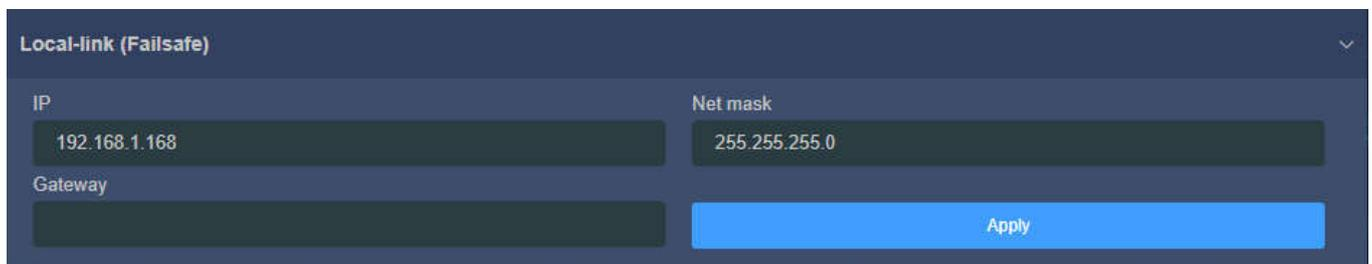
The screenshot shows a configuration window titled "Local-link (Failsafe)". It contains three input fields: "IP" with the value "192.168.1.168", "Net mask" with the value "255.255.255.0", and "Gateway" which is currently empty. A blue "Apply" button is located at the bottom right of the configuration area.
