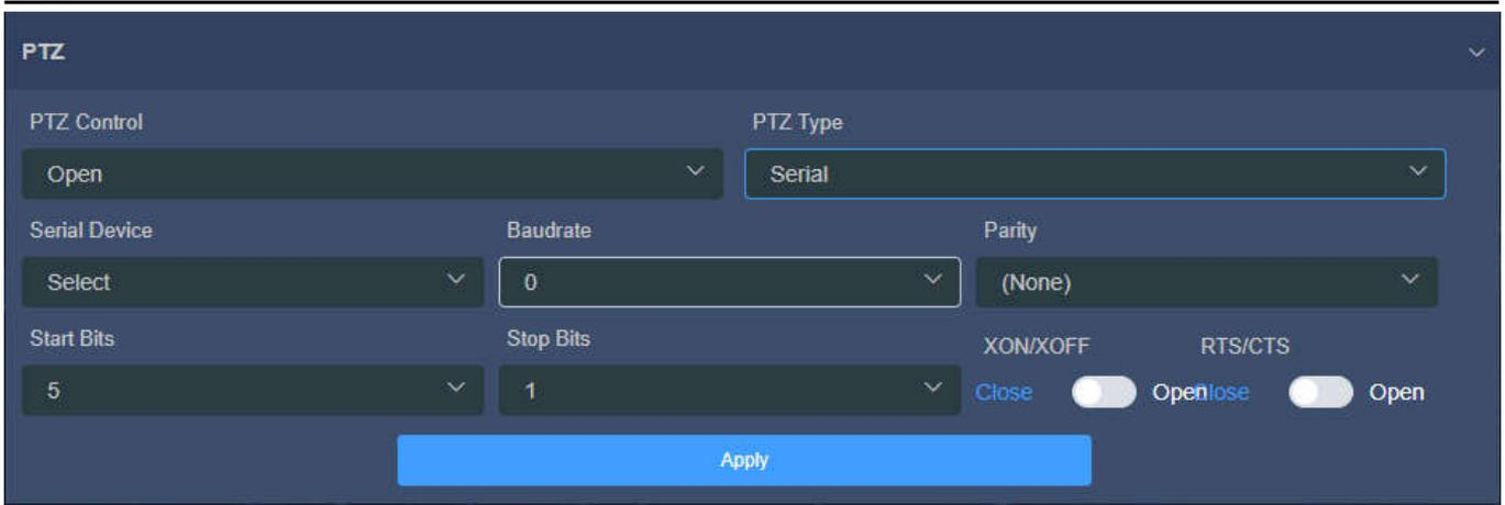
After configuring the control parameters correctly, PTZ control service can be realized by PTZ control panel of NewTek Studio Monitor.
