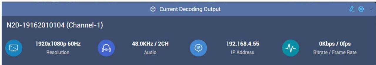
If the current decoding source is disconnected, a warning notice will be displayed at the up-right corner showing the device is offline.
