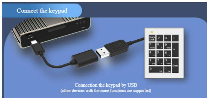
Press **【NumLock】** on the keypad, if the light is on, you can operate the decoding switch. Press 1~9 to select the corresponding 1~9 preset decoding source, and press 0 to select blank output.
