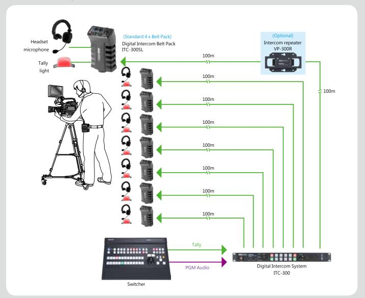
The Datavideo ITC-300 is an 8-channel single wired communication system, featuring power, intercom and tally signal over Ethernet to belt pack. The video director can select to talk to an individual channel or to all channels simultaneously.
