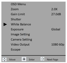
2. After that, you can press the "MENU" button which is located on the rear panel of the BC-15P camera to enter the sub-menu which is shown in the following diagram. After that, you can adjust your desired White Balance mode (Auto, Indoor, Outdoor, and One-push) by the "Up-Arrow button" or
