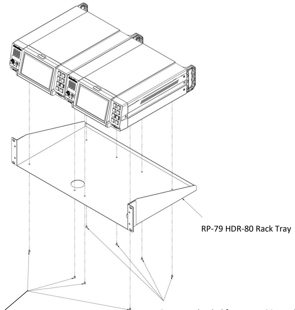
Four screws in the product package used for securing the HDR-80 front to the rack tray.
