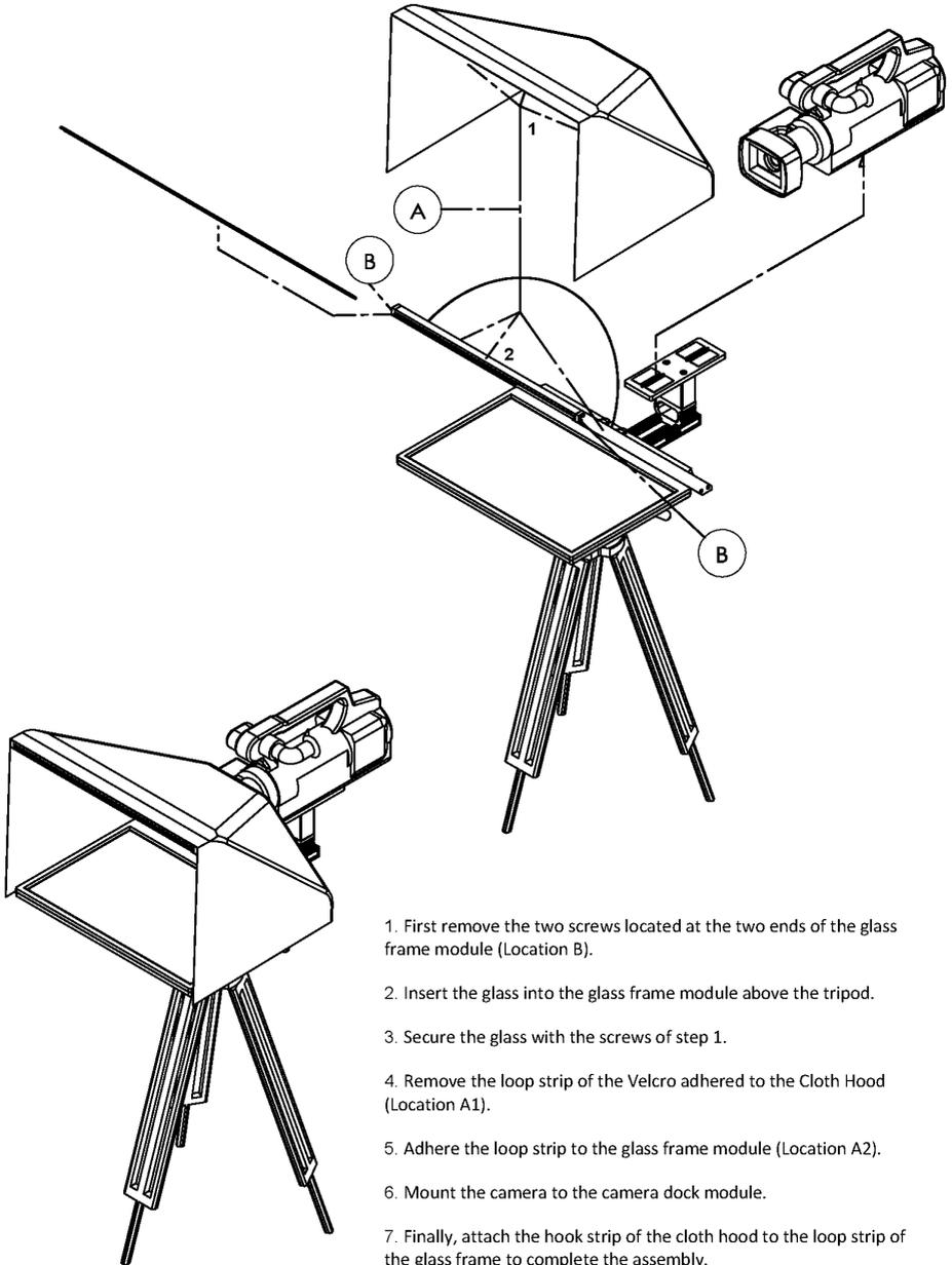
1. First remove the two screws located at the two ends of the glass frame module (Location B).
