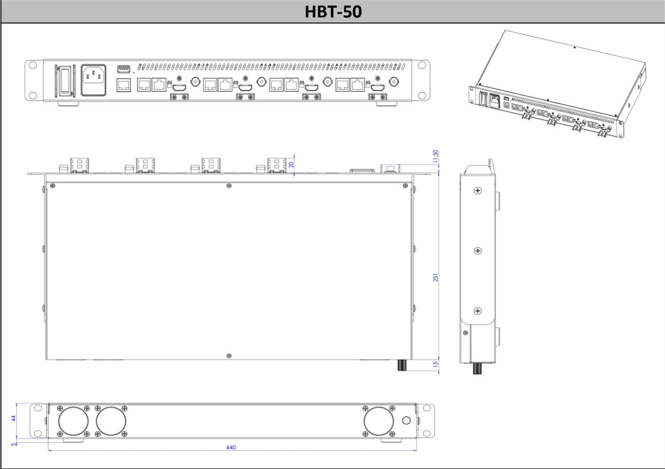
All measurements in millimeters (mm)
