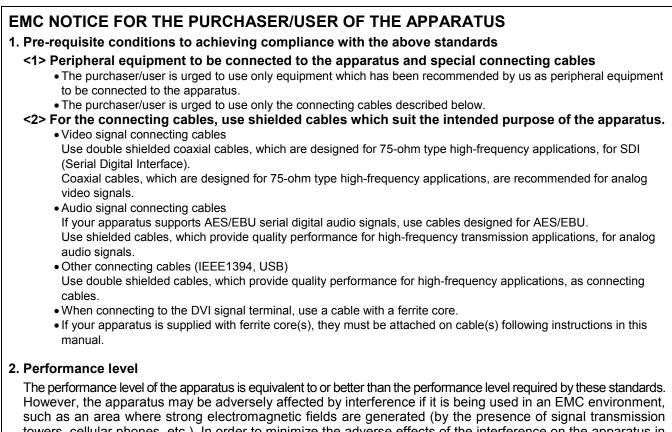
towers, cellular phones, etc.). In order to minimize the adverse effects of the interference on the apparatus in cases like this, it is recommended that the following steps be taken with the apparatus being affected and with its operating environment:
