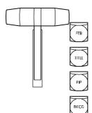
A short column of buttons positioned at right beside the fader lever determines what video layers (see Section 10.1.2) are affected by *Cut*, *Auto*, and *Fader lever* operations.
