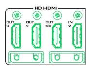
**HD-HDMI Outputs** Connect external HDMI devices for playback of HD videos.
