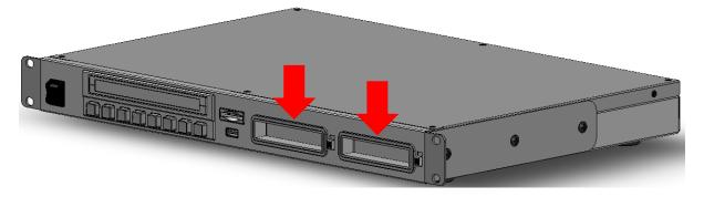
The SSD must be installed in a removable disk enclosure (see <u>Install an SSD drive in a</u> <u>Removable Disk Enclosure</u>) before inserting into SSD slots. After disk insertion, make sure the drive is locked to avoid unintentional disk removal. Move the latch to the LOCK position. To remove the disk, unlock the drive then pull the disk out of the slot.
