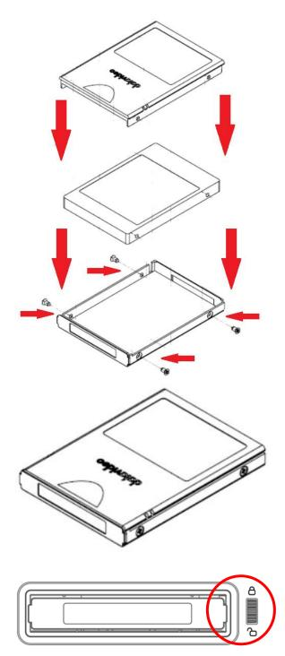
2. As shown in the diagram on the left, place an SSD in the drive enclosure then re-secure the top plate of the drive enclosure using the four screws removed earlier.
