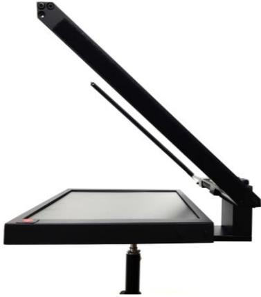
7. You can now fit the lower part of the ENG Prompter Frame **item B** to your tripod or light stand using one of the three 3/8 threaded holes, use the 3/8 to 1/4 adapter, **Item P** if required. Typically, the central 3/8 hole provides the correct balance if not using a talent monitor, the front 3/8 hole should be used with a talent monitor.
