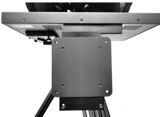
3. If your monitor has a 100MM VESA mount, first attach the VESA adapter plate, **item T** to the vertical mounting rail, **item S** using the 12mm M4 screws, **Item CC**, then attach the monitor to the VESA adapter plate using the 8MM M4 screws, **item CCC**.
