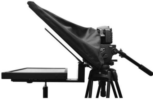
10. Position the TP-700 in front of the camera lens and pull the draw cord to secure the cloth Snood / Hood, **item I**, around the camera lens and to shut out light from the camera side.
