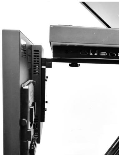
2. If your monitor has a 75MM VESA mount, attach the monitor directly to the vertical mounting rail, **item S** using the 14mm M4 screws, **item U**.
