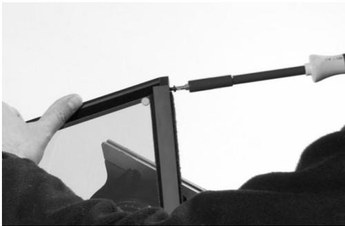
5. Optionally, secure the glass sheet within the frame using the small M4 screws, **item U**, at the top of each frame slot.
