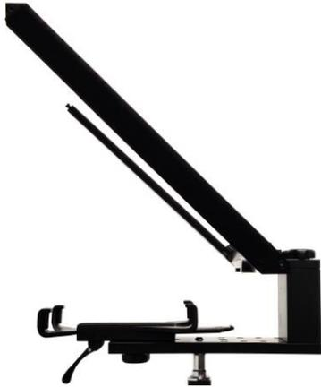
7. You can now fit the lower part of the ENG Prompter Frame **item B** to your tripod or light stand using one of the three 3/8 threaded holes, use the 3/8 to 1/4 adapter, **Item P** if required. Typically, the central 3/8 hole provides the correct balance.
