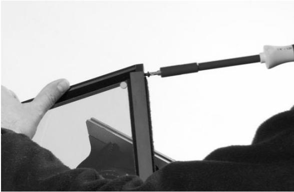
7. Optionally, secure the glass sheet within the frame using the small M4 screws, **item U**, at the top of each frame slot.
