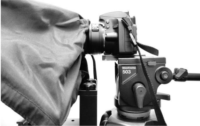
10. Position the TP-650 MKII in front of the camera lens and pull the draw cord to secure the cloth Snood / Hood, **item I**, around the camera lens and to shut out light from the camera side.
