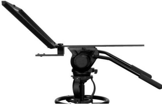
5. Slide the Glass frame, **item G**, on to the front of the TP-650 MKII ENG prompter rail, **item A**. Ensure the upper part of the Glass Frame, **Item G**, is leaning away from the camera position and secure with the two wing nut screws, **item H**.
