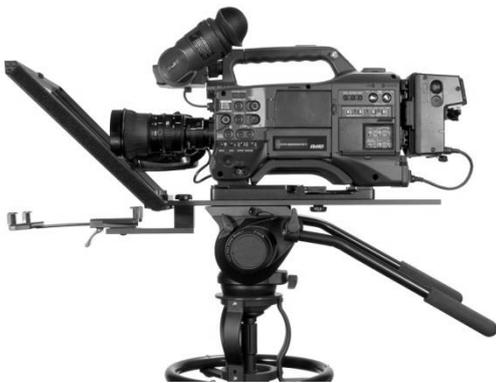
11. You can now mount the ENG camera to the tripod adapter plate. **Take care** to protect the camera lens and the 70/30 mirror glass. If necessary slide everything further along the prompter frame.
