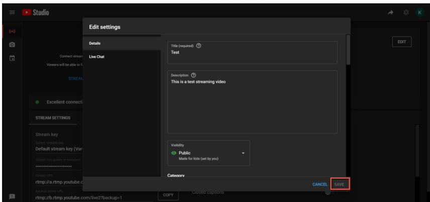
5. Users can see the Stream Key and Stream URL that are provided by the Youtube streaming platform. Please copy the stream key and stream URL and then paste them into the “**First Stream MRL**” within the “**Network**” option of the PTC-285 Web UI. Please click “**On**” and please check the checkboxes of “**Audio**” and “**Video**”.
