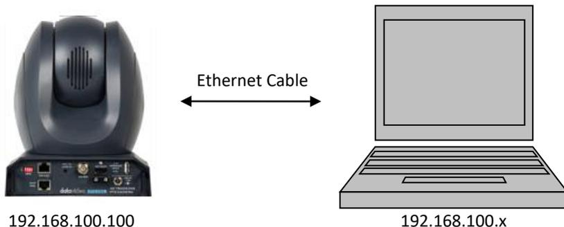
On your PC/laptop, open a web browser and in the address bar, enter the camera's default IP address, 192.168.100.100 then press the **ENTER** key which should take you to login page of the web interface.
