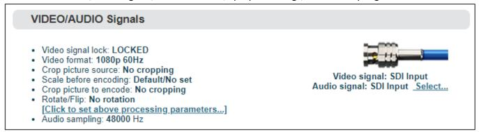
If "video signal lock" displayed as "no signal (display blue screen)", it means the video input source is not detected by the device. Please check if the input cable is plugged in. If "Audio sampling" is displayed as "OHz", the audio signal is not collected on the device. Please check if the audio of the input source is normal.
