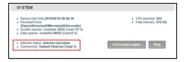
Note: Please confirm whether USB 4G card enables dial-up connection function, SIM card is workable, otherwise the network maybe unavailable. Users can insert a USB 4G card into a computer to test whether it can provide Ethernet access function.
