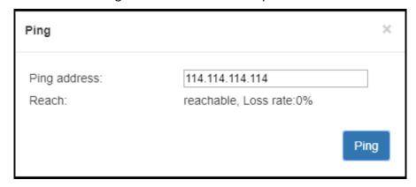
Note: If Ping public IP address is reachable, but Ping domain name is unreachable. Generally, it is because the DNS server configuration is incorrect.
