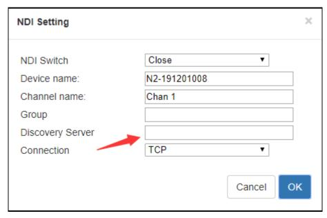
Install NDI tools on the receiving end and open "NDI access manager". Click to enter the "advanced", cancel the "multicast sending enabled" function, select "Use discovery server", and set the "Server IP" address to the IP address of your computer that enables the discovery server function. After configured, the receiving end can discover the NDI stream registered with the server.
