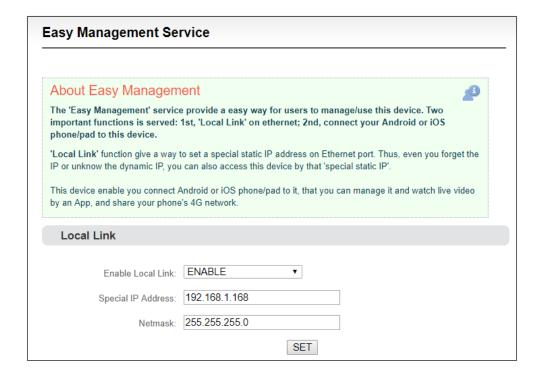
"Local Link" is to bind the encoder to a separate IP address, this IP address does not affect the use of other network cards, in special cases, it can play a role to manage encoder, this address can be manually changed, the default address is 192.168.1.168.
