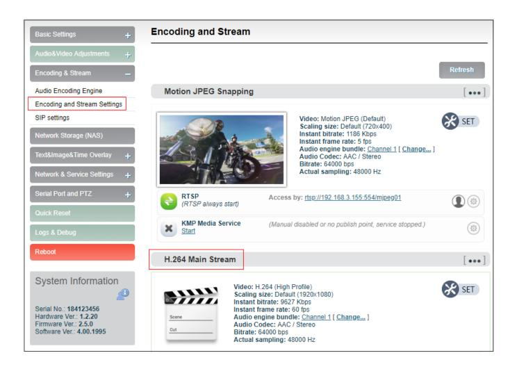
Note: For NDI, the sub-stream of the encoder must always be in the running state, otherwise it may cause the NDI stream to have no audio.
