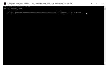
NDI encoder configures the receiving IP address in the discovery server, and NDI will be registered with the server. It is recommended that the receiving address should be configured as a static IP address to prevent the loss of NDI connection due to IP reallocation.
