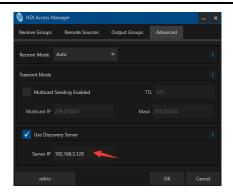
Note: after this function is enabled, the mDNS auto discovery function is invalid. The stream of the decoder can only be sent to the specified server, and the receiver end must register with the same discovery server to pull the NDI stream.
