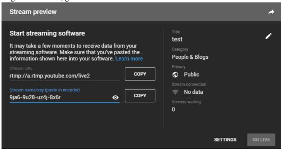
Streaming point should be like Server URL+Stream name/key, for example: rtmp://a.rtmp.youtube.com/live2/9ja6-9u28-uz4j-8x6r
