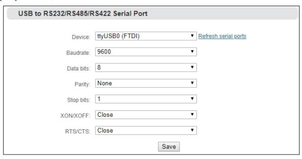
Note: The encoder can automatically identify the USB serial port conversion device of universal USB to Serial/FDTI chip/PL2303 chip. If the USB to RS232/RS422/RS485 converter (line) you inserted cannot be recognized and the converter chip is not supported by default, please replace the serial line.
