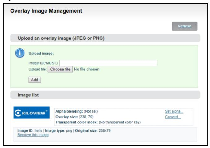
You can change the parameters after uploading the image Set alpha blending: Value range is 0-255, 0 is full transparent and 255 is no alpha blending. Convert:
