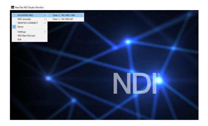
Note: After opening the selected video of the encoder by Studio Monitor, click in the lower right corner of the player to open the Web page of the encoder directly, which is convenient for the management of the encoder.
