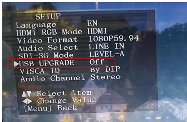
9. Please move the “Microjoystick”
