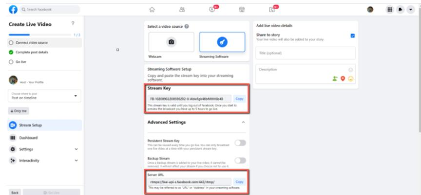
5. Please click the “Copy” buttons which are located next to the “Server URL” and “Stream Key” columns respectively. After that, please paste them to the “First Stream MRL” column in the “Network” option of the PTC-285T web UI.
