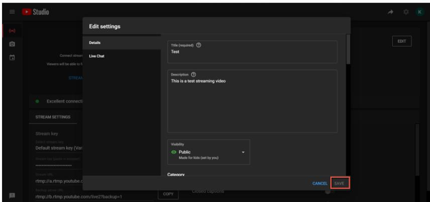
5. Users can see the Stream Key and Stream URL that are provided by the Youtube streaming platform. Please copy the stream key and stream URL and then paste them into the “**First Stream MRL**” within the “**Network**” option of the PTC-285T Web UI. Please click “**On**” and please check the checkboxes of “**Audio**” and “**Video**”.
