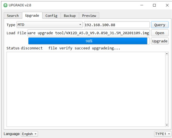
10. After the firmware upgrading is finished, the PTC-285T camera will reboot automatically, please click the “OK” button and then the firmware upgrade procedure is completed.
