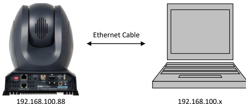
On your PC/laptop, open a web browser and in the address bar, enter the camera's default IP address, 192.168.100.88 then press the **ENTER** key which should take you to login page of the web interface.
