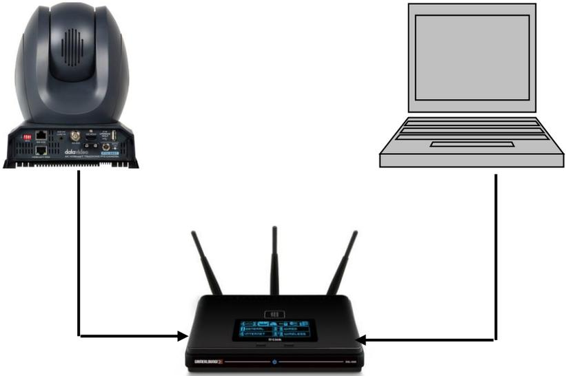
In order to enable the DHCP mode of the camera, please select “Dynamic IP Address” from the “IP Configuration Type” drop-down menu for assigning a dynamic IP address to PTC-285T by the router. After that, please click the “Apply” button to save the new settings and then please reboot the PTC-285T.
