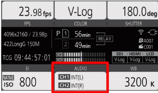
Assignment of audio channel and setting of audio source.
