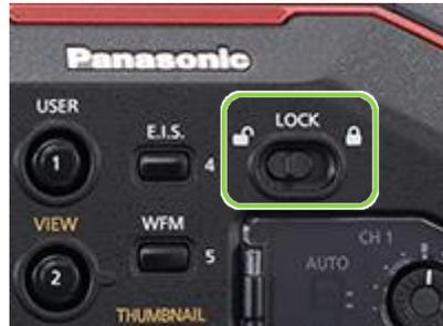
LOCK switch located at left side of the unit
