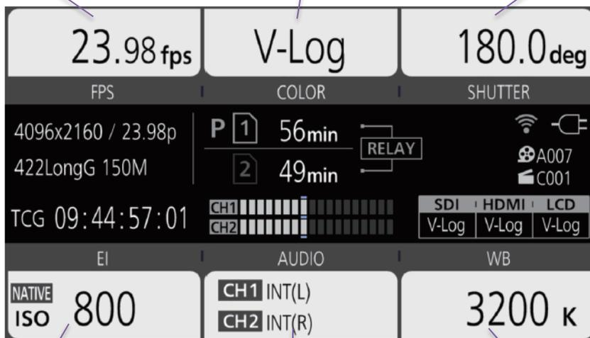
EI (Exposure Index), display mode (ISO/dB) can be switched at MENU > EI > MODE
