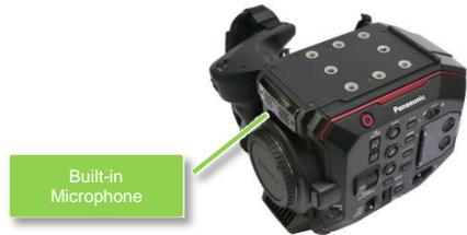
3. Set audio record level knob. To use automatic level adjustment, set the AUTO/MANU switch to “AUTO”.
