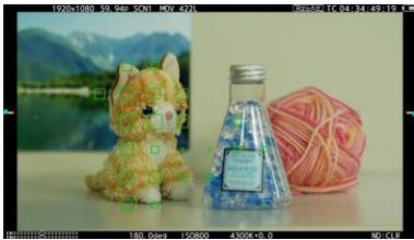
Green square boxes are displayed on the viewfinder image, whose size increases as the object behind the box comes into focus. Adjust focus ring/control so that size of the boxes over the subject/area of interest become maximum. It can be used in combination with “PEAKING” focus assist mode.
