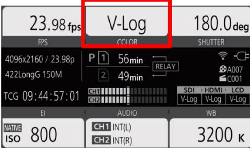
On the AU-EVA1, settings of Gamma & Gamut is called "COLOR". Image COLOR to be recorded can be set in the MAIN COLOR screen. COLOR settings for SDI, HDMI, and LCD output can individually be set.
