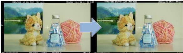
Makes focusing easier by opening aperture (i.e. by making depth of field shallower). Brightness of the image is maintained even when aperture is opened with automatic shutter speed control.
