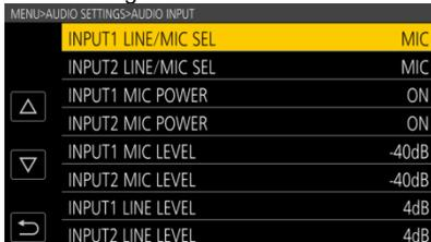
Set to “ON” when the microphone requires +48V power supply from the EVA1.
