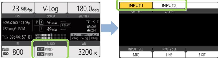
3. Set INPUT1 SEL to MIC and INPUT2 SEL to MIC for audio level.
