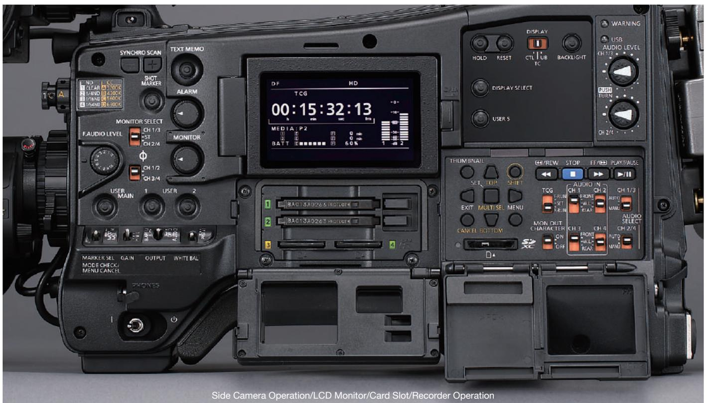
Side Camera Operation/LCD Monitor/Card Slot/Recorder Operation
