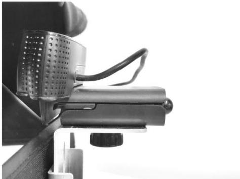
6. Optionally attach your small box camera or web camera to the aluminium camera bracket (**Item B**) using the small 1/4 screw and 1.5mm rubber washer (**Item F**) if required. The position of the camera can be adjusted by loosening screws **C**
