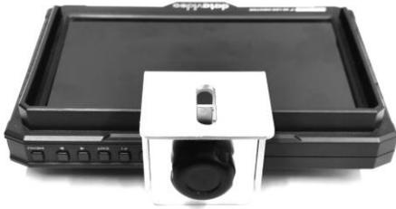
If you intend to mount a small box camera or webcam directly to the TTL-100, attach the aluminium monitor bracket (**Item A**) and the aluminium camera bracket (**Item B**) to the TLM-700 monitor using the large 1/4 screw (**Item D**).
