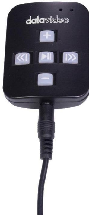
**NOTE:** When using this remote in wired mode the **DV Prompter Plus app** should also be set to **Wired – WR-500** in the **Remote menu option**.
