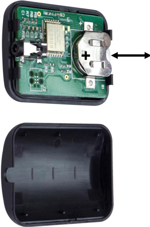
This button battery can be replaced by the user when it dies. **Please remove the case back carefully** to avoid user damage to the PCB or case. Then slide the old battery out.
