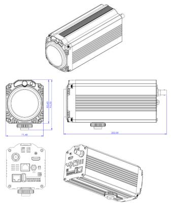
All measurements in millimeters (mm)
