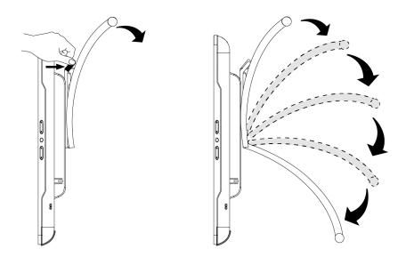
Removing and installing the Smooth Tilt Stand You can remove the interactive pen display from its stand.
