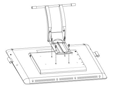
3. Align the four holes in the stand with the mounting holes in the back of the interactive pen display.
