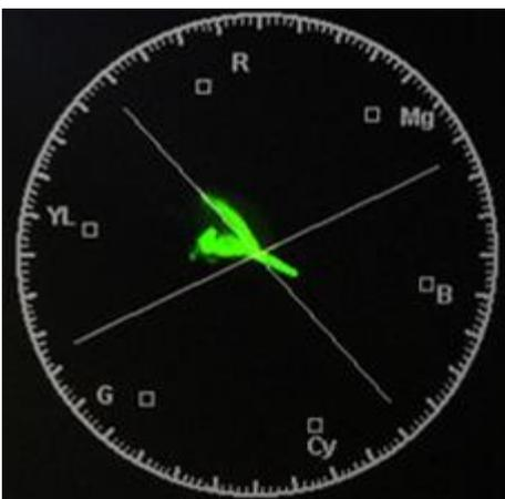
The vector scope is used to measure the color information such as **Hue** and **Saturation** in a video image.
