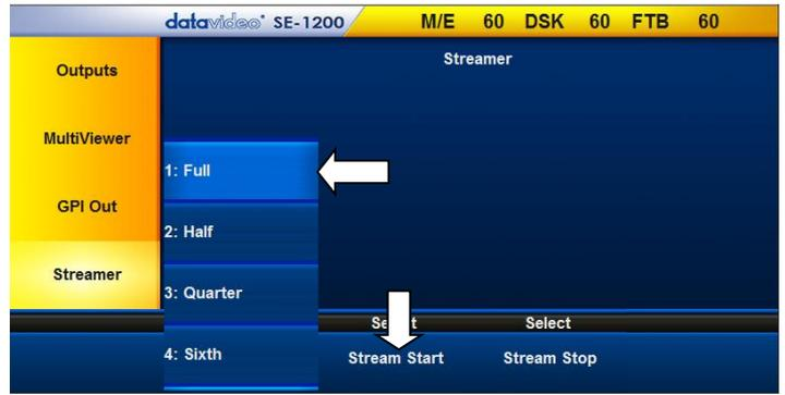
By choosing **HALF** instead of **FULL** you are using less bandwidth to support the multi view stream being sent across the IP network (no audio is sent across the IP network). Reducing the size of the multi view stream may also help overcome delay/latency issues over the network.
