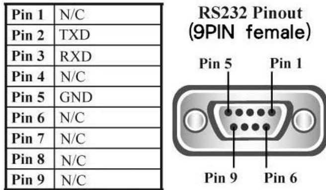
The user may establish the RS-232 connection between RMC-260 and SE-1200 MU using a male-to-male cable with the wiring scheme as depicted in the diagram below.
