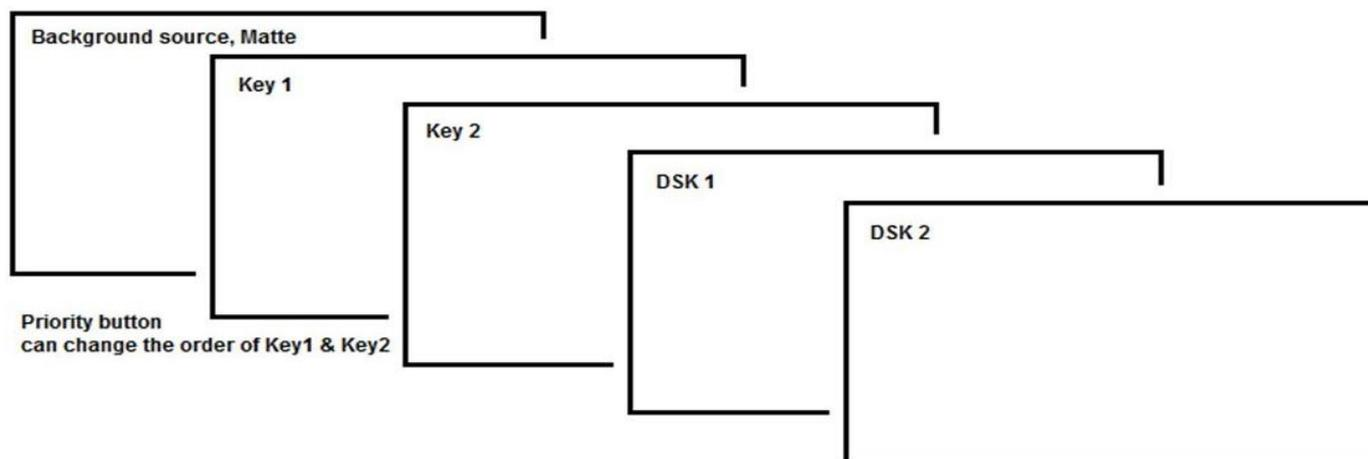
Before attempting to use the SE-1200 MU's PIP, Chroma, Luma and Down Stream Keying functions, it may help to first understand the order of the video layers at the SE-1200 MU Program outputs.
