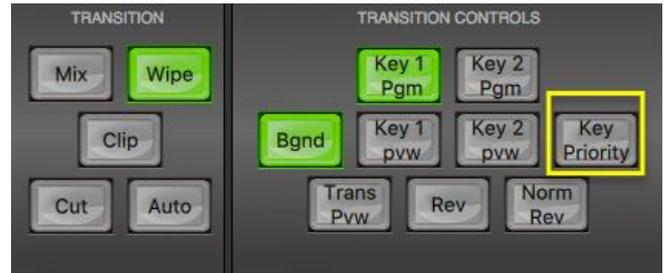
When Key 1 and Key 2 are both active in Preview (or Program), they may overlap each other on the screen. Using the Priority Button you can change the order of these keyers. The button acts in a toggle on/off way, i.e. Key1 over Key2 or Key2 over Key1.
