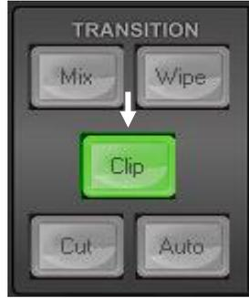
To change the rate of transition for the **Auto** button press the **Home** menu button and change the **M/E Trans** duration value in frames.
