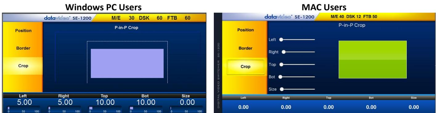
The **Left, Right, Top** and **Bottom** edge values of the crop can be adjusted individually or together using the **Size value**. Click on a single value to adjust just that edge of the PIP.
