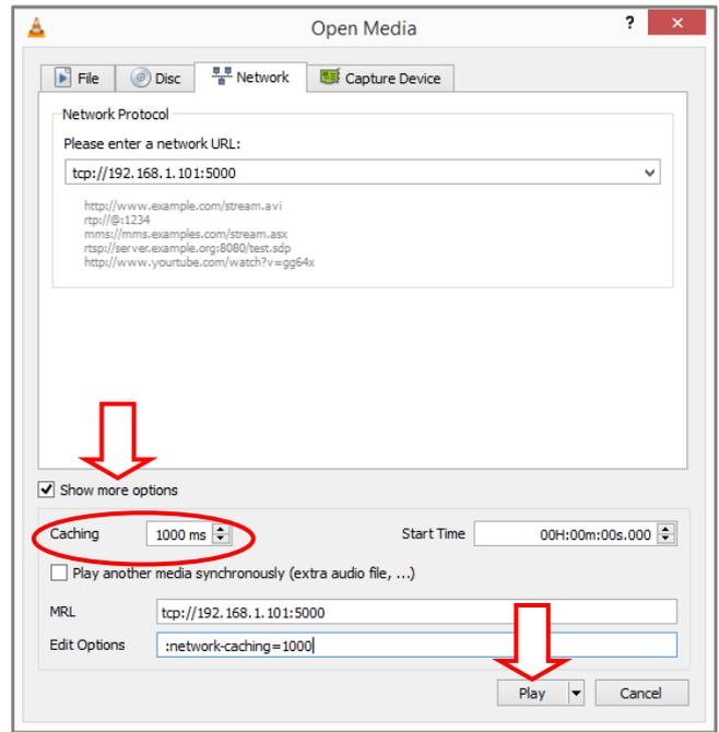
**Note:** The VLC caching value and multi view stream size are also related to latency. Reducing the SE-1200 MU streamer size may also help reduce the multi view delay or latency across the IP network. The quality of the multi view image will also be affected by these settings.
