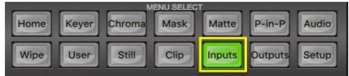
2. Six video input channel selection buttons will be displayed. **Click on the input channel button that you wish to Freeze.**
