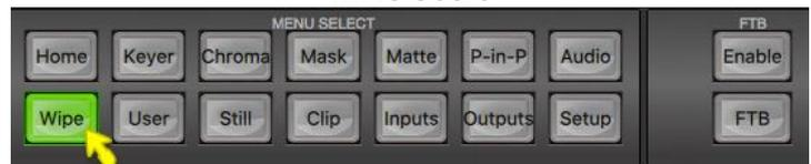
Each wipe pattern consists of blue and white colors. The white represents the current Program image (A) and the blue represents the WIPE-IN image (B). There are a total of 32 WIPE presets offered by the SE-1200 MU as shown below.
