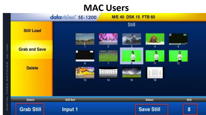
5. Click **Grab Still** to capture the freeze image from the SE-1200 MU's Program output into working memory.
