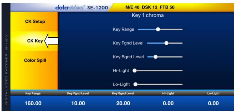
The **CK Key** parameters and values are shown along the bottom of the display. The respective sliders are shown in the diagram.
