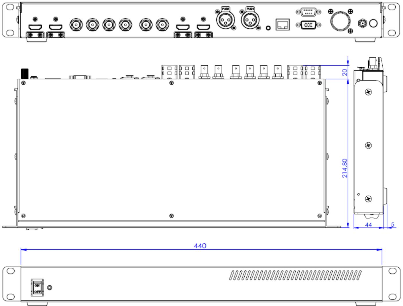
All measurements in millimetres (mm)
