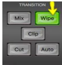
To change the rate of transition for the **Auto** button press the **Home** menu button and change the **M/E Trans** duration value in frames.
