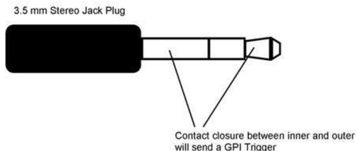
This GPI socket can also be used as a socket to trigger record or playback events with other equipment such as the Datavideo HDR-70 recorder.
