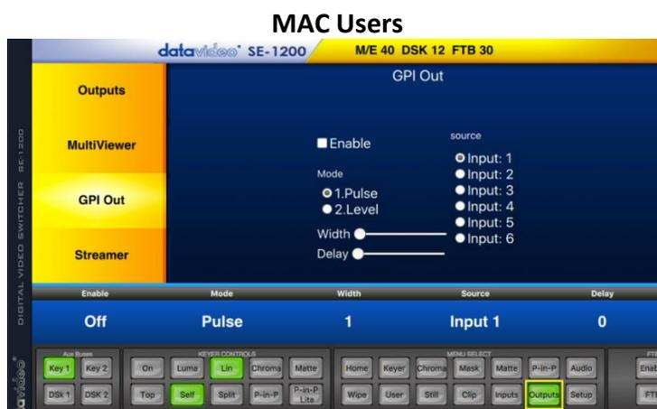
After turning **On** the GPI **Enable**, select the GPI **Mode**, which is either set as **Level** or **Pulse**. The GPI signal **Width** can also be configured by setting a value (1~9).
