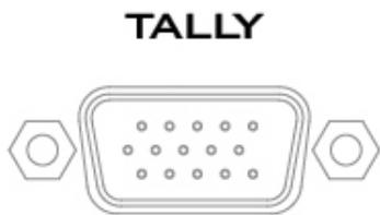
The SE-1200 MU has a D-sub 15 pin female tally output port. These connections provide bi-color tally information to a number of other Datavideo products, such as the ITC-100 eight channel talkback system and the TLM range of LCD Monitors. The ports are open collector ports and as such do not provide power to tally light circuits.
