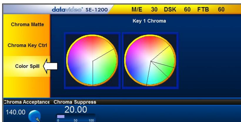
The **Color Spill** parameters and values are shown along the bottom of the display below. These settings are used to control/remove any unwanted Chroma or color Spill from the background onto the foreground subject. There are two sectors drawn on the **Chroma** palette, one represents the wider **Chroma Acceptance** range and the narrower **Chroma Suppress** range.
