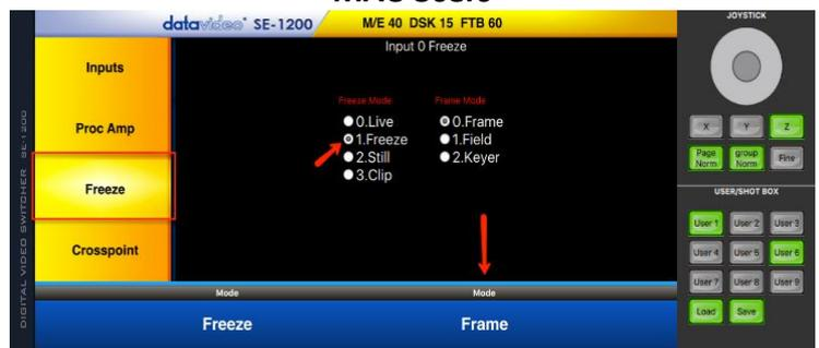
4. The Freeze Mode located at the bottom right of the screen can be set to a full **Frame** or one **Field**. In most cases **Frame** should be used.
