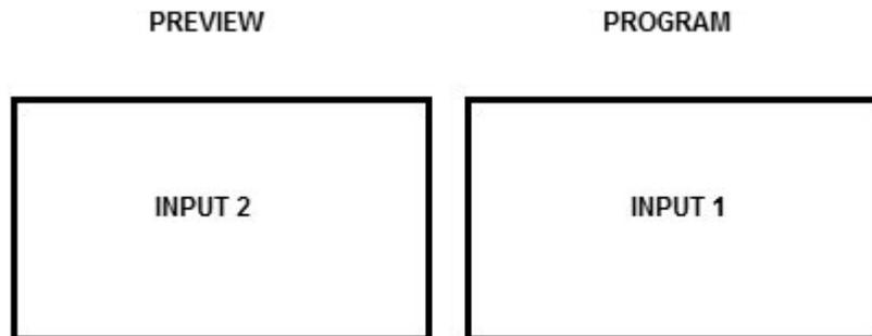
Using the **TRANSITION CONTROLS panel** click to select the **Trans Pvw button** (back lit green is ON). Next select and apply the transition or wipe that you would like to test on the Preview monitor.
