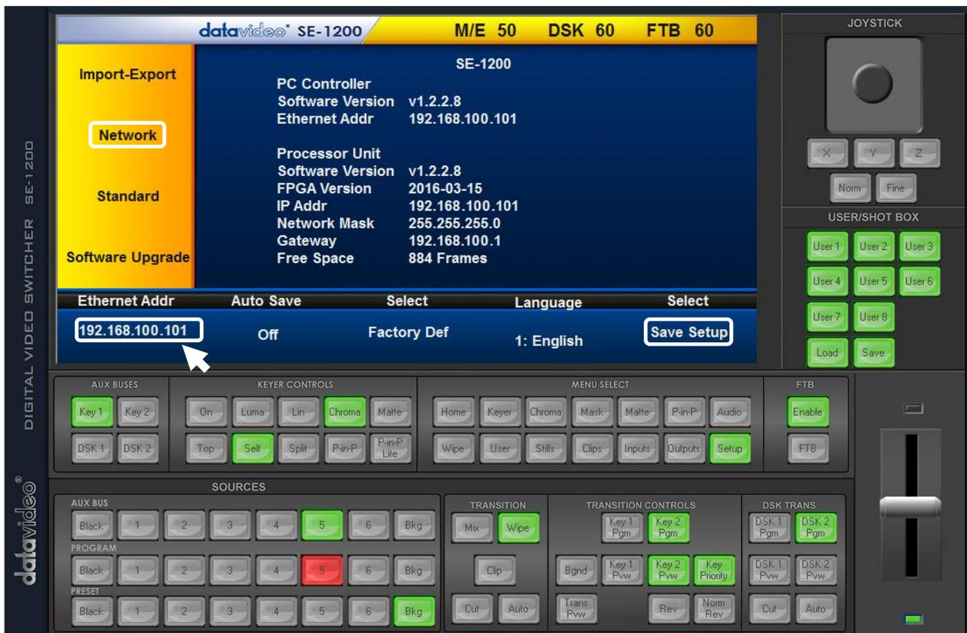
**Ethernet Addr** – This is the target IP address i.e. the location on the local network, or the internet, where the software can talk to the SE-1200 MU. By clicking **Ethernet Addr** you can enter a new address, once entered click **Enter**. The next time the software controller is opened, it will try to contact the switcher on this new Target IP address.
