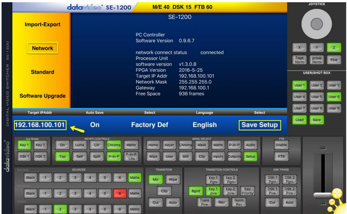
**Target IP Addr** – This is the target IP address i.e. the location on the local network, or the internet, where the software can talk to the SE-1200 MU. By clicking **Target IP Addr** you can enter a new address, once
