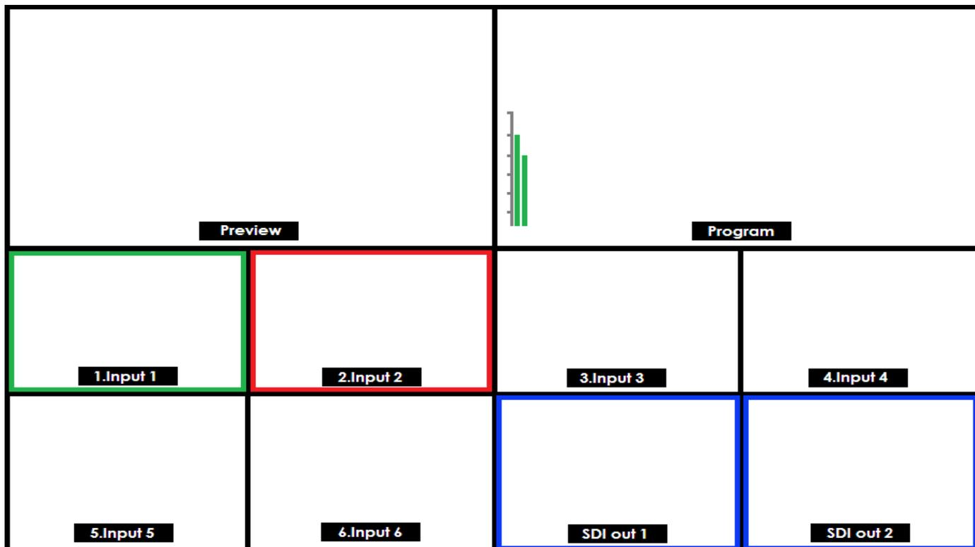
The SE-1200 MU multi view output can be supplied locally, from either the HDMI1 or SDI outputs 1 and 2 on the unit's rear panel, see [section 2.2](#) (Chapter 2). The multi view can also be streamed over a LAN/internet connection, see [section 3.2.2](#) (Chapter 3).
