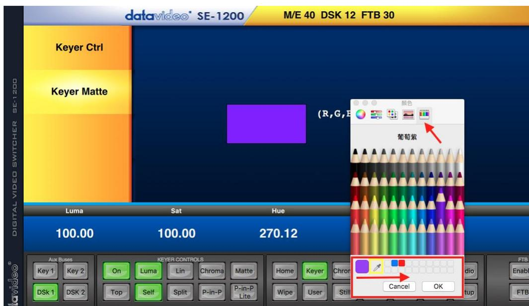
Finally, select the pencil of the color that you need. Below the pencils, the color selected will be shown at the leftmost end in a square box. To save the selected color, drag it to one of the smaller square boxes to the right.
