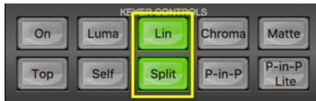
**Step 3:** The **Split** button is backlit green, select the CG key source on the **AUX BUS Row** (input 3).
