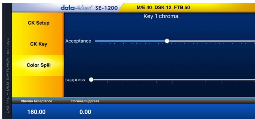
The **Color Spill** parameters and values are shown along the bottom of the display below. These settings are used to control/remove any unwanted Chroma or color Spill from the background onto the foreground subject. There are two parameters in the **Color Spill** option, which are **Chroma Acceptance** and **Chroma Suppress**.
