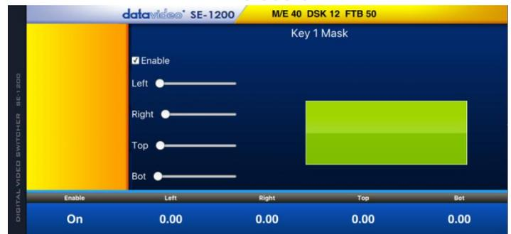
3. The **Left, Right, Top & Bottom** values allow the user to set the inside **Left, Right, Top & Bottom** edges of the keyer mask.
