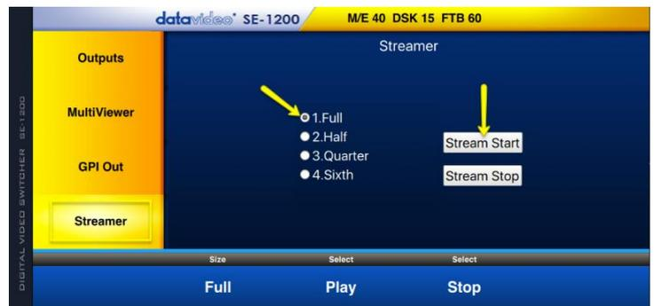
By choosing **HALF** instead of **FULL** you are using less bandwidth to support the multi view stream being sent across the IP network (no audio is sent across the IP network). Reducing the size of the multi view stream may also help overcome delay/latency issues over the network.
