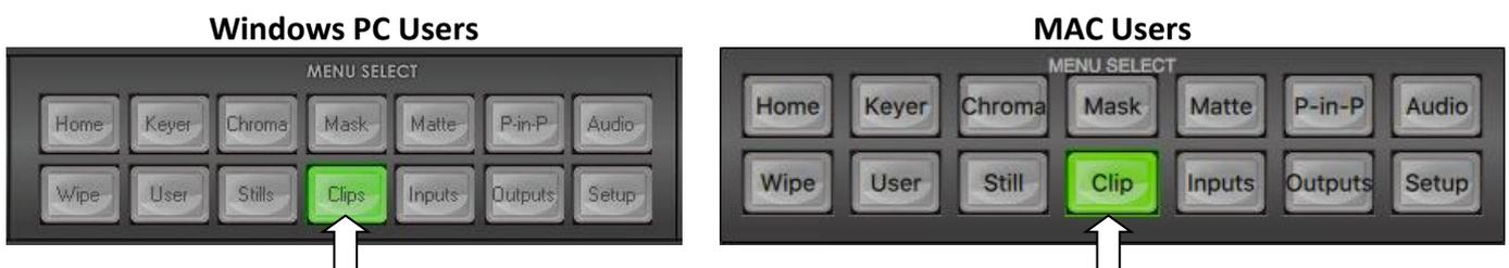
To load the clip, simply click on the **Clip** option and then select **“Load Clip”**. The clip is always loaded to input 6 so anything loaded to input 6 before will be replaced by the clip.
