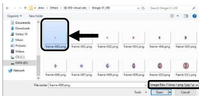
Click **Open** to start the clip import. If your files are not the .pic format, they will be automatically converted to .pic format by the **Switcher Image Import/Export utility** first.
