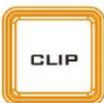
Press the **Clip** button to enable the Clip (Stinger) transition mode.
