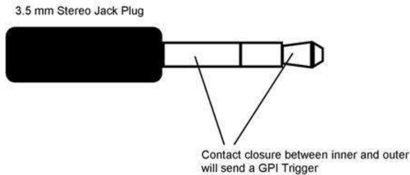
This GPI socket can also be used as a GPO socket to trigger record or playback events with other equipment such as the Datavideo HDR-80 or HDR-90 recorder.
