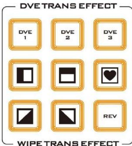
There are 32 different 2D WIPE effects and 3 different 3D WIPE effects to choose from when using the SE-2600 switcher. To select a different WIPE transition, either select a WIPE style in the **TRANS EFFECT** area of the SE-2600 Control Panel or the **Start** Item of the OSD Menu (see the table below). Before you make the selection, make sure the **TRANS BG** and **WIPE/DVE** buttons are enabled.
