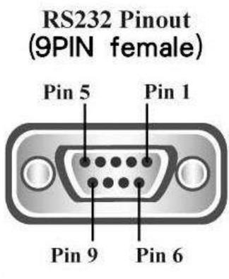
The diagram shows a 9-pin D-sub female connector. The pins are arranged in a 3x3 grid. The top row contains Pin 5 (left) and Pin 1 (right). The middle row contains Pin 9 (left) and Pin 6 (right). The bottom row contains two unlabeled pins. The connector is labeled "RS232 Pinout (9PIN female)".
