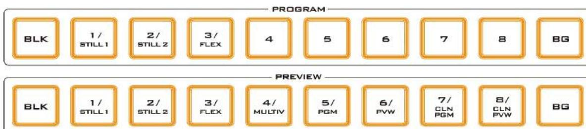
This row of buttons is typically used to select the switcher's Preview or Next source output image. The selected source will be **backlit Green** on this row. You can transition between Preview and Program using the **T-Bar**, the **CUT** button or the **AUTO** button.
