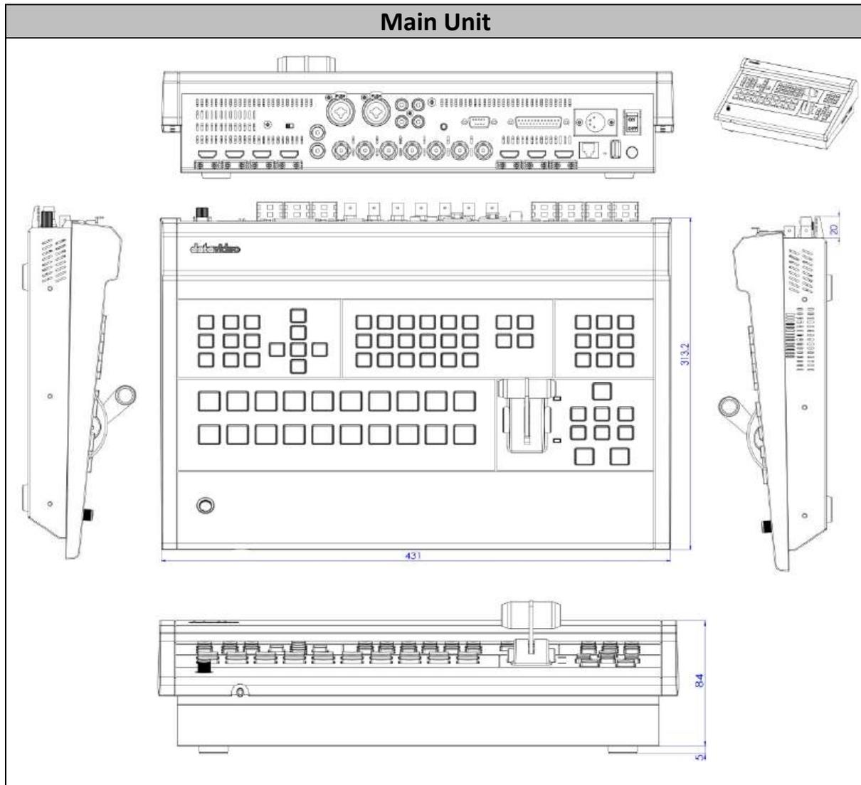
All measurements in millimeters (mm)
