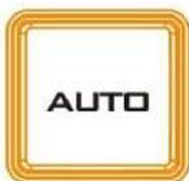
The **AUTO** button is used instead of the manually operated **T-Bar** and automatically performs the complete selected transition between Program and Preset over a set period. The **M/E** value in the **START** menu is used here. See [Section 4.1](#).
