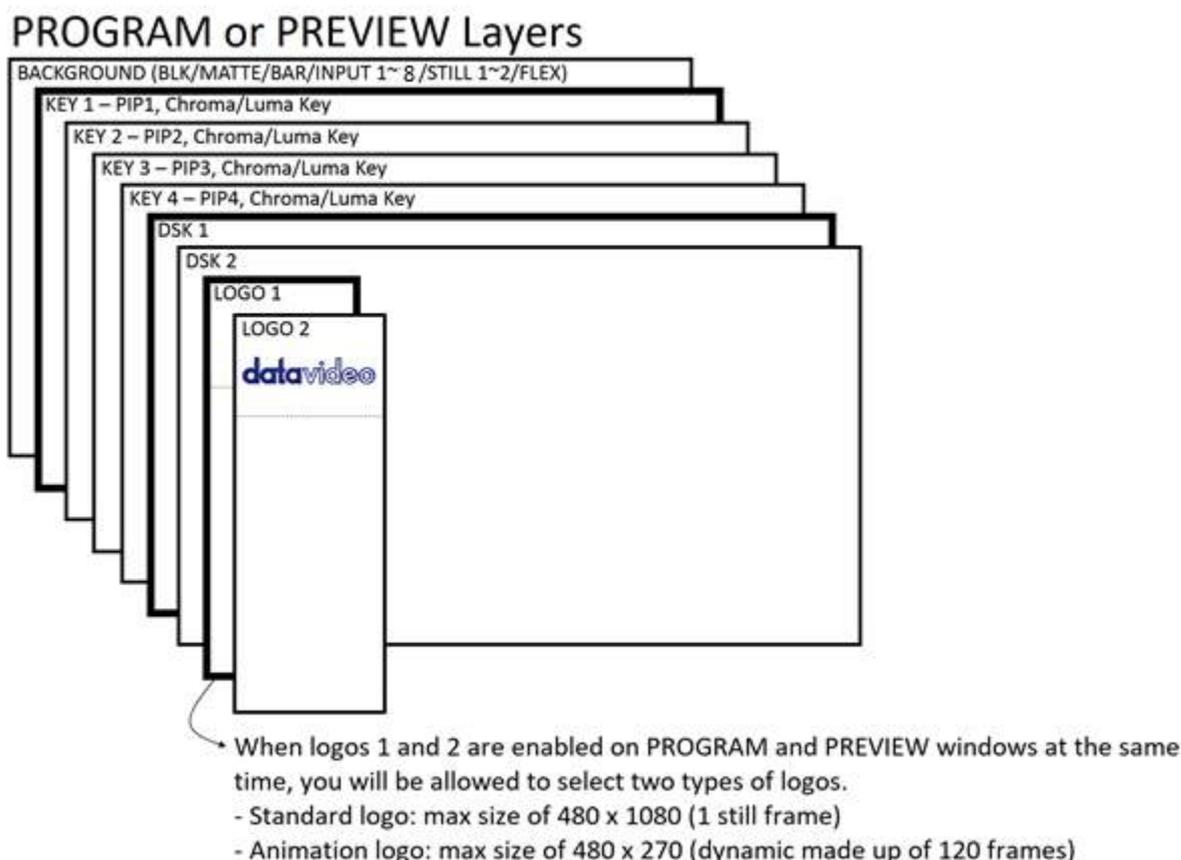
The **Background video layer** is the normal video layer (**black screen, color matte, color bars, inputs 1-8, still pictures 1 and 2 or Flex™ sources**) when mixing and switching with the SE-2600. It occupies the whole screen area of the Program output. This layer can be hidden or partly hidden by the PIP, DSK and LOGO layers in front of it.
