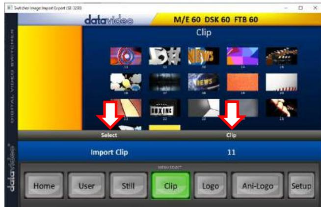
**Tip:** The **Switcher Image Import/Export** utility does the conversion from bmp/png/jpg to the .pic file format automatically. All you need to do is to give the utility a starting file location and it will give the utility an idea where to start linking all images up into a sequential animation file.
