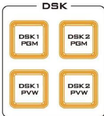
On the SE-2600 Control Panel / Keyboard there are four DSK keys. These are labelled Program and Preview. The upper DSK1 and DSK2 keys relate to activating Down Stream Keying on the Program outputs. The lower DSK1 and DSK2 keys relate to activating Down Stream Keying on the Multi-view or Preview outputs.
