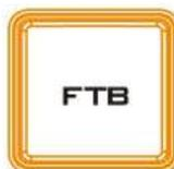
The **FTB** button (Fade To Black) fades the current video program source to black. When pressed again it acts in reverse from complete black to the currently selected program video source. To set the transition time, open the OSD menu, then the Start menu, and modify the FTB value accordingly.
