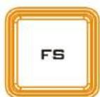
The SE-2600 has eight video channels and each of these channels has its own Frame Store, making a total of eight Frame Stores. Each of these Frame Stores can hold one still image. The FS button allows the user to call the still image into the production and toggle between that still image of the Frame Store and the live video input connected to that same video channel.
