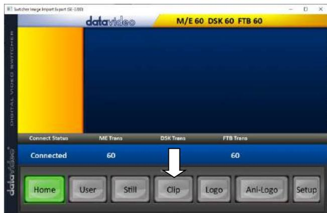
The clip number allows you to select a location where you can save the clip. To import a clip from the computer into the SE-2600, select **Import Clip**.
