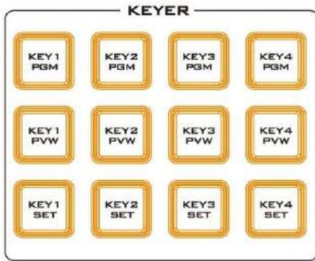
On the SE-2600 Control Panel / Keyboard there are eight **KEYER** keys. These are labelled Program and Preview. The upper **KEYER** keys relate to activating Picture-In-Picture images on the Program outputs. The lower **KEYER** keys relate to activating Picture-In-Picture images on the Multi-view or Preview outputs. Before activating Picture-In-Picture images on the output image, you should first set these **KEYER** keys to PIP mode.
