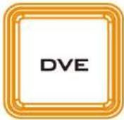
The **WIPE/DVE** button is selected when a 2D wipe or a 3D DVE transition between the selected Program and Preset sources is required. This WIPE or DVE transition effect is produced by then moving the **T-Bar** manually or by pressing the **AUTO** button. Select 2D WIPE in **OSD menu** → **Start** →
