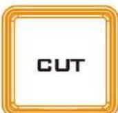
The **CUT** button is used to immediately switch between the currently selected Program and Preset sources.
