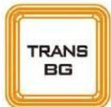
Turning on the **TRANS BG** button allows you to activate the MIX, WIPE or Stinger transition with the background image/video.
