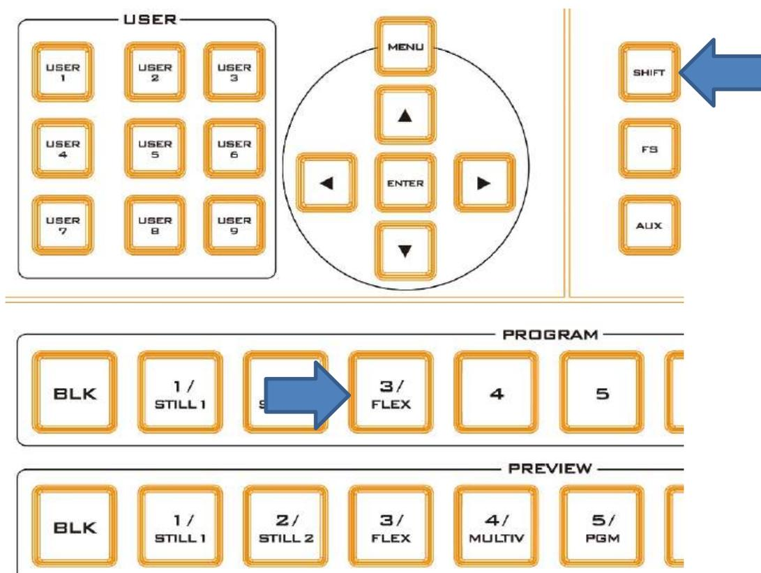
2. Press the **MENU** button on the switcher's control panel to open the OSD menu on the Multiview screen and select **Flex Src** sub menu. On the sub menu that opens, select any of the presets to enable the desired preconfigured layout on the screen.
