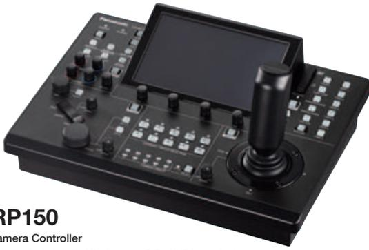
A ZOOM/FOCUS rocker mounted on the joystick manages pan and tilt operations for zoom and focus control and intuitive single-handed operation. The built-in touch display allows for easy and quick operation of all essential camera functions.
